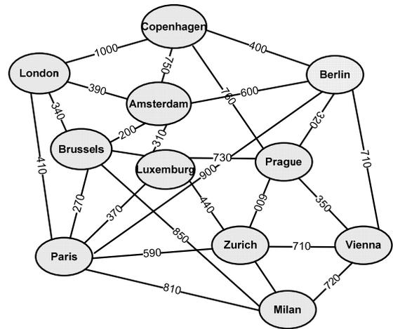
Fig. 2: Pan-European test network COST 239
