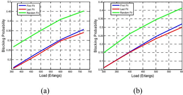
Fig.3 Network performance for the three backup path wavelength assignment schemes under different loading conditions (a)  $\lambda=60$  and  $\mu=6,8,10,12$  (b)  $\mu=10$  and  $\lambda=30,40,50,60$
