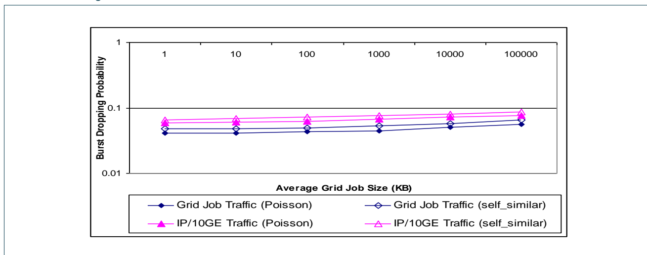
Figure 63: Average Burst Dropping Probability under Varying Average Grid Job Sizes
