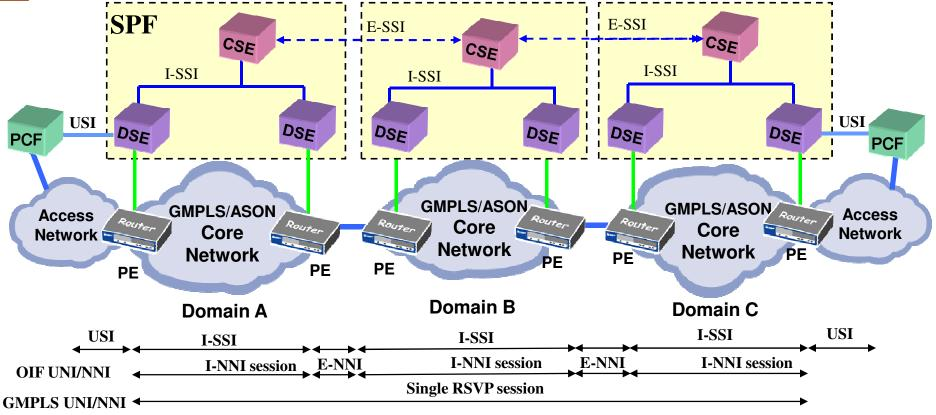
OIF UNI/NNI = several RSVP sessions → external coordination for each domain is needed for end-to-end service provisioning GMPLS UNI/NNI = single RSVP session → external coordination among the end points is needed for end-to-end service provisioning (e.g., for obtaining bidirectional connections)
